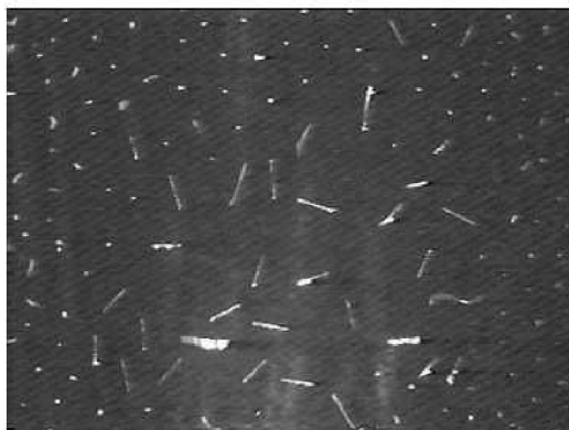
FIG. 1. Top view on rodlike particles levitating in a rf sheath (from Ref. [13]). Dots at the periphery are vertically oriented “short” rods ( L=300 \text{ }\mu\text{m} ); “long” particles ( L\geq 600 \text{ }\mu\text{m} ) levitate horizontally in the center.
